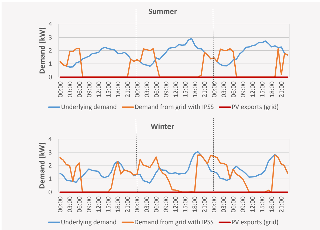
Figure 17 Forecast impact of IPSS on daily load of a large consumer in New South Wales around times of regional maximum demand
